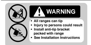
If you pull the range out and away from the wall for any reason, make sure the Anti-Tip bracket is engaged when the range is pushed back against the wall.
